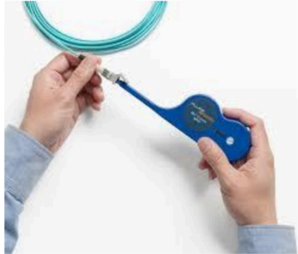
Optical Connector Cleaning Tool
