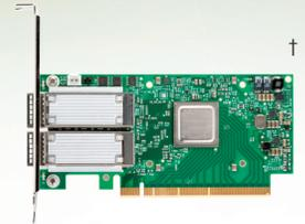
ConnectX-5 with Virtual Protocol Interconnect<sup>®</sup> supports two ports of 100Gb/s InfiniBand and Ethernet connectivity, sub-600 ns latency, and very high message rate, plus PCIe switch and NVMe over Fabric offloads, providing the highest performance and most flexible solution for the most demanding applications and markets: Machine Learning, Data Analytics, and more.
