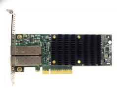
T6225-LL-CR runs at a higher clock rate and provides the best sub micro-second end-to-end latency, while offloading the host CPU from a variety of typical storage, networking, and cloud related protocols. This will enable savings in host CPU acquisition costs, power and operational costs, and dramatically increases system performance.
