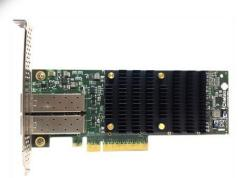
T6225-CR provides sub micro-second end-to-end latency, while offloading the host CPU from a variety of typical storage, networking, and cloud related protocols. This will enable savings in host CPU acquisition costs, power and operational costs, and dramatically increases system performance.
