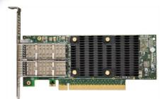
and in addition adds support for integrated offload of IPsec, TLS/SSL, DTLS and SMB 3.X crypto.
