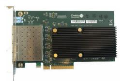
The fifth-generation (T5) technology from Chelsio provides the highest 10GbE performance in the industry and dramatically lowers host-system CPU communications overhead with on-board hardware that offloads TCP/IP, iSCSI, FCoE and iWARP RDMA processing from the host system and frees up host CPU cycles for other applications. As a result, the system benefits from higher bandwidth, lower latency, and reduced power consumption.
